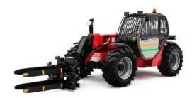
For easy manoeuvring in mines, the MT-X 733 has a turning radius of 3.72 m. and a high ground clearance (45 cm).
